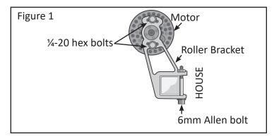
Parts Supplied: Roller Bracket assembly
